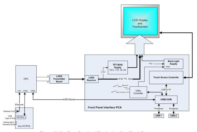
Figure 13-17: Front Panel and Display Interface Block Diagram
